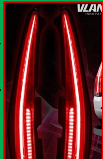
Recommended "Repair" Adding inward LED Bulb Strip
